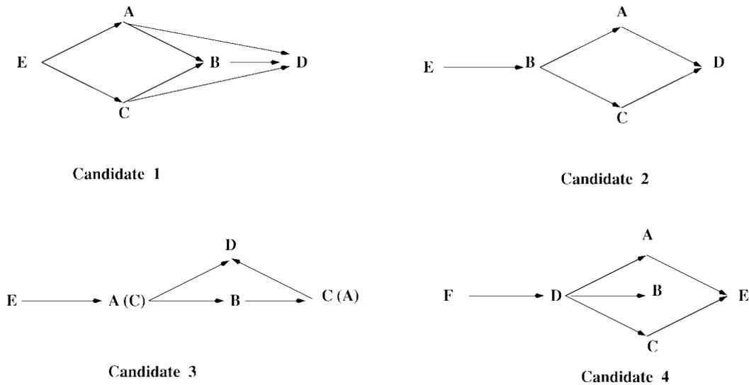
Fig. 11. Datum flow chains representing different location logics.
