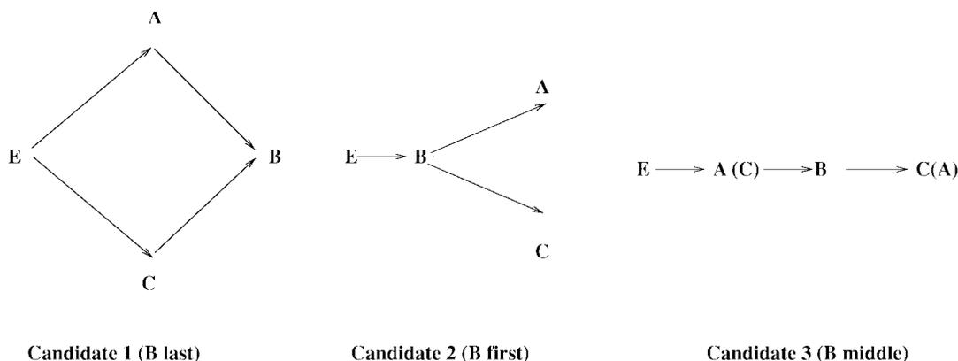
Fig. 4. Datum flow chains representing different location logics.
